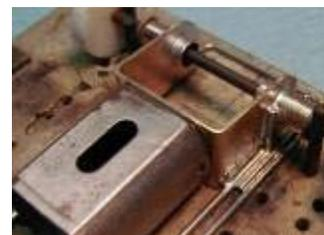
12. Now let's work up front. I use a non-rotating axle, cut from a 2 7/8" long piece of .093 piano wire, and polished until it shines. I mount it in position in the jig at the chosen wheelbase (usually somewhere between 3 7/8" and 4") with jig wheels to get the necessary front end clearance. 4 pieces of .055 wire, bent 90 degrees are used to hold the axle:
