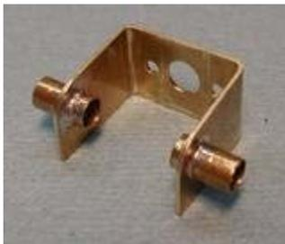
2. I cut a nosepiece from .062 brass plate that is as wide as the bracket, and 1" long. I use 1" wide strip for this. Scribe a center line along the length of the nosepiece to help with alignment later.
