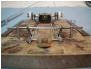
13. Bumpers: These are the parts for the well-known "Pepe" bumper, invented by Philippe de Lespinay back in the 1970's. This is a system that works well to prevent major damage to the other pieces of the car by being the first parts to give way in a wall shot. All made from .062 wire.
