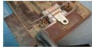
15. Front hinge tubes: These are cut 3/4" long from a piece of 1/16" outside diameter brass tubing. Cut 8 at a time, as they will be used for the pin tubes too. Put a drop of oil inside each tube before soldering them in position to ensure the tubes do not fill with solder. Two tubes go up front against the bumper,
