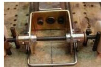
11. Now you can add the outer rails, using a piece of .055 wire to space them away from the inner rails. Solder the rails to the bracket brace and to the opposite side of the axle tube from the inner rail.
